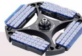
PCR Swing-bucket rotor for 12 × 8 PCR strips 0.1/0.2 mL or 4 × 1/4 twin.tec PCR plate 96, unskirted divisible or 96 × PCR tubes with 0.2 mL spins up to 3,217 × g/6,000 rpm (S-96 × 0.2-PCR)
