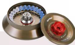
Aerosol-tight Eppendorf QuickLock® rotor for 24 × 1.5/2.0 mL tubes spins up to 21,330 × g/15,060 rpm; PTFE-coated for increased chemical resistance and easy cleaning (FA-24 × 2-PTFE)
