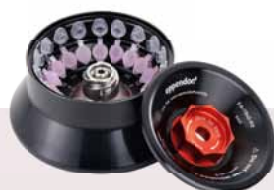
Aerosol-tight Eppendorf QuickLock® rotor for 18 × spin columns and 1.5/2.0 mL tubes designed with an extra high rim to support open tube lids during centrifugation; spins up to 18,565 × g/15,060 rpm (FA-18 × 2-Kit)
